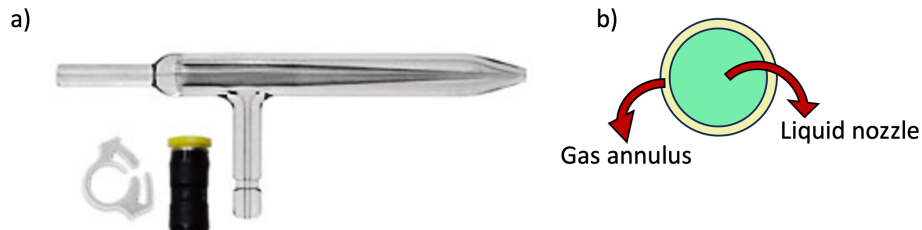
Figure 3. (a) SeaSpray high-performance nebulizer and (b) cross-sectional diagram depicting the nozzle tip showing liquid nozzle and gas annulus.
