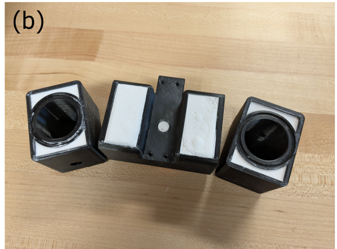
Figure S3: Photos of the assembly process. (a) Photo of the 3D-printed shell before filling with plaster, showing the stainless steel resonator that has been pressed into the shell. (b) Photo after filling with plaster but before glue-up; note that an error with the 3D printer caused the central microphone port to break through during assembly in (b), but the port and o-ring groove typically appears as in (a) even after filling.
