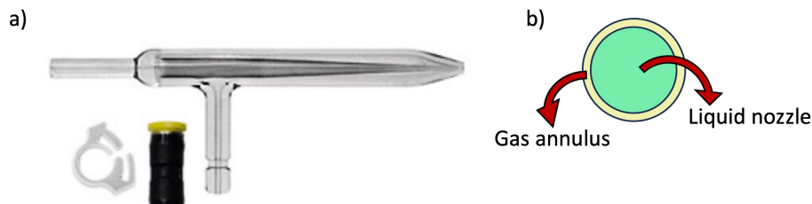
Figure 1. a) SeaSpray high performance nebuliser, b) cross-sectional diagram of the nozzle tip showing liquid nozzle and gas annulus.
