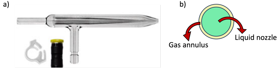
Figure 3. a) SeaSpray high performance nebuliser, b) cross-sectional diagram depicting the nozzle tip showing liquid nozzle and gas annulus.
