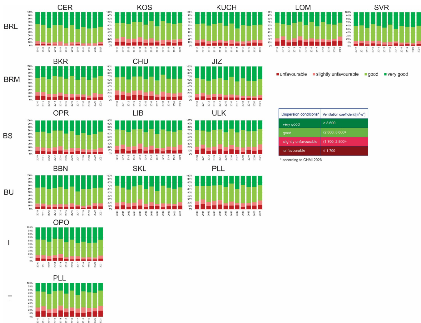
50 Figure S3: Dispersion conditions evaluated by ventilation coefficient value according to method CHMI (2026) at individual stations 2011–2021.
